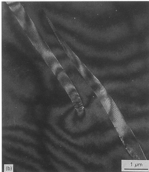
Figure 4 Transmission electron micrographs: (a) experiment 7, P_i = 84 GPa, bright field showing the numerous open fractures; (b) experiment 2, P_i = 34 GPa, weak-beam micrograph showing the microcracks (evidenced by their Moiré pattern) in a pristine matrix.
