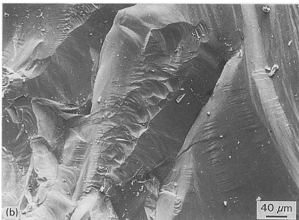
Figure 2 Scanning electron micrographs of laser-induced craters. (a) General view, experiment 5, P_i = 34 GPa. (b) Experiment 3, P_i = 34 GPa: larger magnification; note the hackle morphology.
